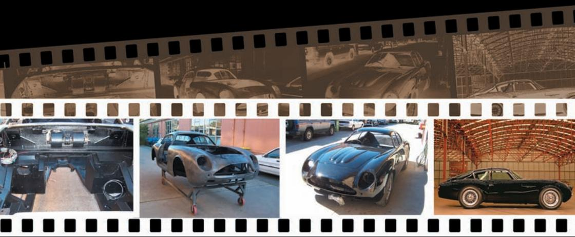
The DBSZ concept is powered by an uprated version of the 4-litre 6 cylinder Aston Martin Vantage engine with DB4 GT specification pistons and camshafts and coupled to a 5-speed synchromesh manual gearbox. It is also available in V8 form, utilising a DBS/V8 model platform and drivetrain. A choice of either automatic or 5-speed manual transmissions can be offered.
